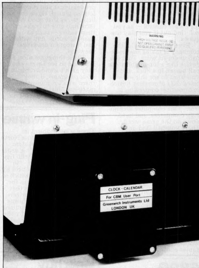
Greenwich Instruments has put a battery in the clock it has developed for the PET, to avoid the clock stopping each time the computer is turned off.
